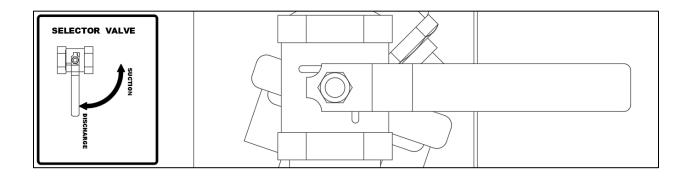
7. OPEN THE AIR SUPPLY VALVE. THE PRESSURE READING SHOULD INCREASE TO 5-7 PSI.
