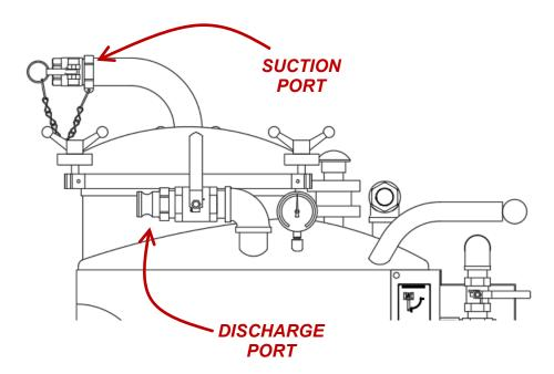
YOU ARE REQUIRED TO SUPPLY AIR CONNECTIONS THAT FIT YOUR AIR SYSTEM. THE SHARKS AIR-LINE TERMINATES IN ½" NPT PIPE THREAD. THE SHARK REQUIRES A MINIMUM 3/8" DISCONNECT; (½" FOR OPTIMAL PERFORMANCE). ¼" BLOW-OFF CONNECTIONS ARE TOO LIMITING ON THE AIR SUPPLY REDUCING PERFORMANCE.
