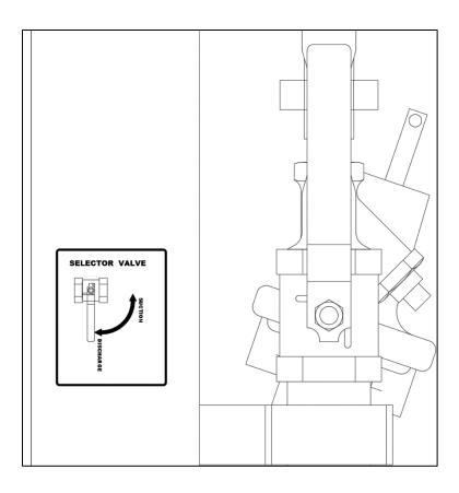
4. OPEN THE AIR SUPPLY VALVE. THE VACUUM READING SHOULD INCREASE TO 20-26" HG.
